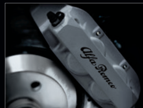
Dual-cast, cross-drilled, self-ventilated, 305- x 28-mm front discs with Brembo® fixed 4-piston calipers
