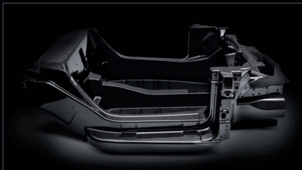
Genuine carbon fiber monocoque chassis
